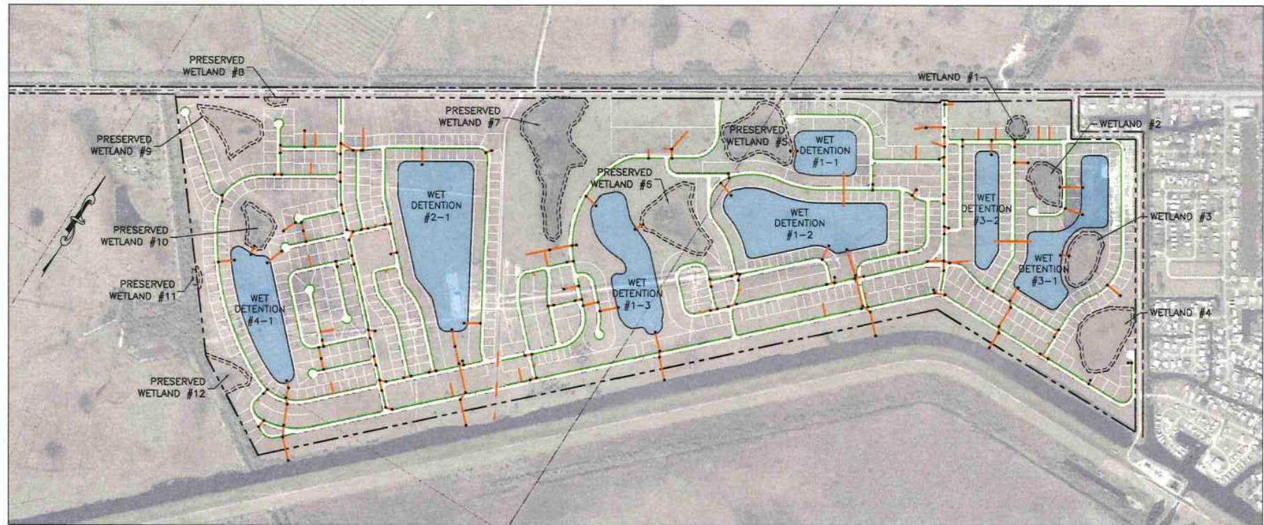
FIGURE 6 STORMWATER MANAGEMENT PLAN LAKEFRONT ESTATES
