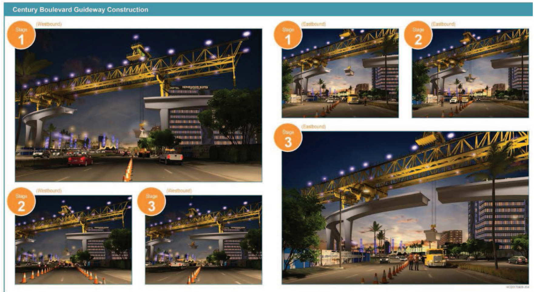
Figure 10-18 LINXS proposal for Guideway construction over Century Boulevard
