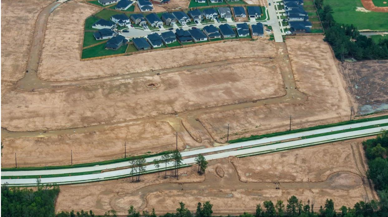
Water, sewer, and drainage improvements and grading are complete and streets have been cut.
